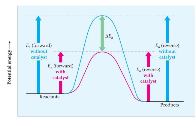
The activation energy for the **catalyzed pathway** (red curve) is lower than that for the **uncatalyzed pathway** (blue curve) by an amount  $\Delta E_a$ .
