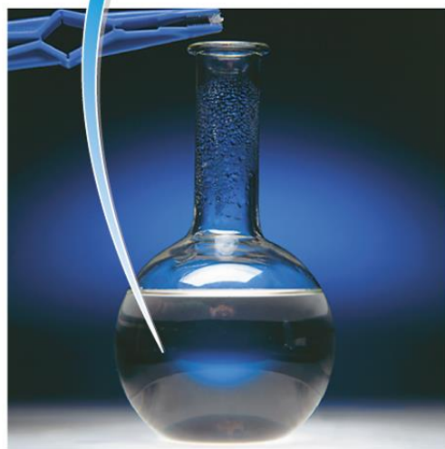
A supersaturated solution of sodium acetate in water.
