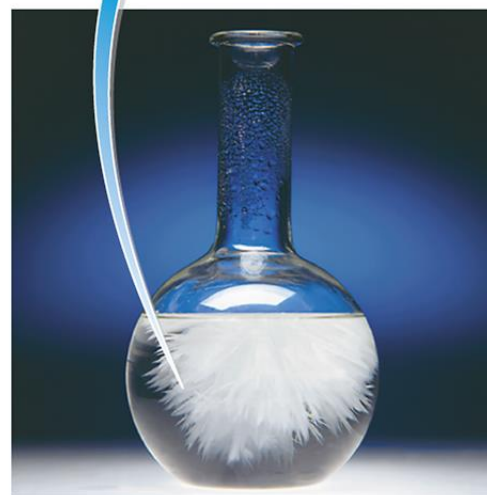
When a tiny seed crystal is added, larger crystals begin to grow and precipitate from the solution until equilibrium is reached.
